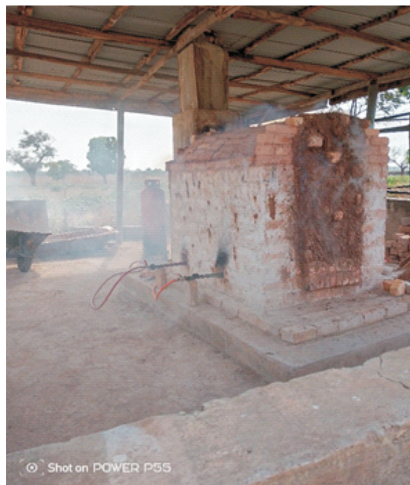
Fig. 8: Firing with the fabricated burners
